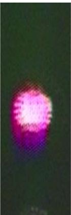
Digitized video image of a 633-nm laser beam reflecting from the polygon scanner. The image was recorded approximately 10 inches from the scanner using an ordinary TV camera.
