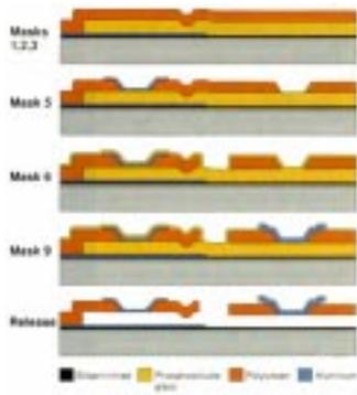
In the surface micromachining process, a sacrificial layer is grown or deposited and patterned, and then removed wherever the mechanical structure is to be attached to the substrate. Then, the mechanical layer is deposited and patterned. (To make more complex structures, additional layers of mechanical and sacrificial materials can be used.) Finally, the sacrificial layer is etched away to release the mechanical structure.
