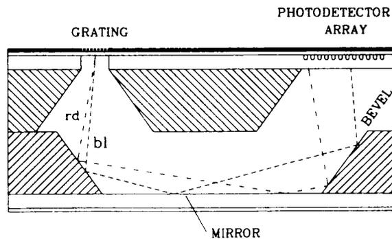
Spectrometer with integrated grating and detector array fabricated in (100) silicon.
