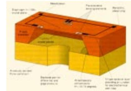
A bulk-micromachined pressure sensor — shown in cross-section — contains a thin silicon diaphragm formed by etching the silicon wafer with alkali-hydroxide. The deflection of the diaphragm depends upon pressure and is sensed by boron-doped piezoresistors.
