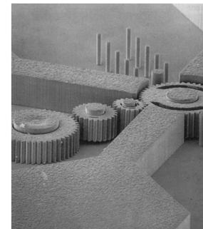
In the sacrificial LIGA technique, a magnetic micromotor and assorted microgears are selectively plated onto a sacrificial layer deposited on a silicon substrate. Afterward, the moving parts are freed by selectively etching and undercutting the sacrificial layer. The structure shown was designed for friction testing, and being approximately 300  $\mu\text{m}$  across, can achieve very high angular velocity because of its low inertial mass.
