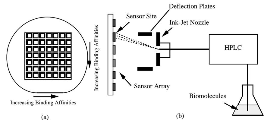
(a) gradient in binding affinities across wafer; (b) system to deposit biomaterial at specific sensor sites
