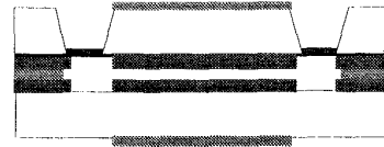
Figure 4. Tunable IR filter using evaporative coated spacers.
