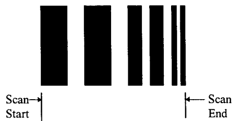
Figure 9: A test bar code with alternating light and dark periods with decreasing bar width and spacing.
