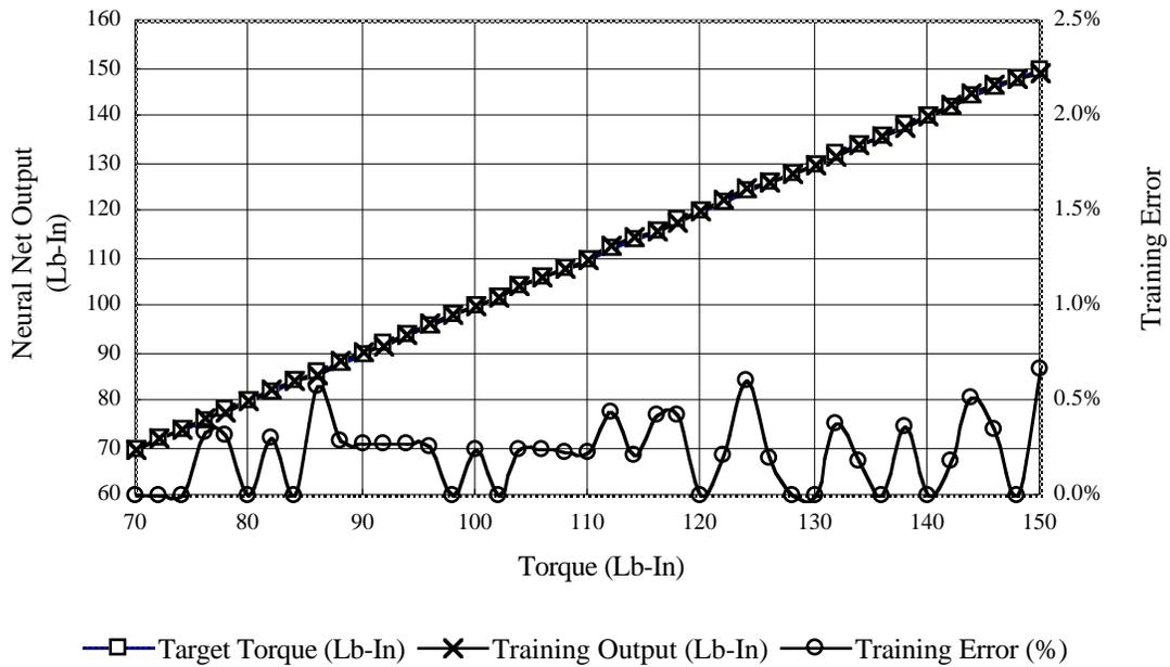
Figure 6. Performance of Neural Net Torque Estimator (Training)
