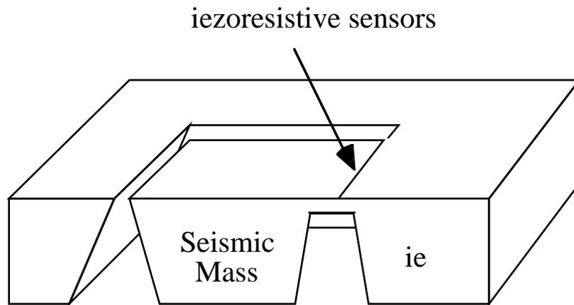
Figure 4. Cross-section of silicon piezoresistive sensor
