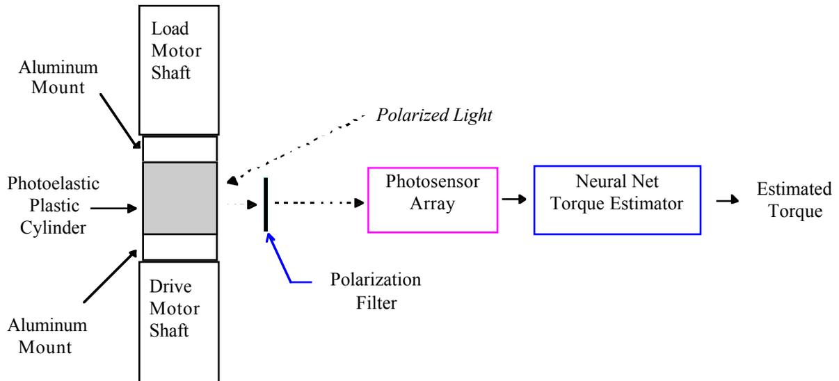
Figure 2. Experimental Torque Sensor
