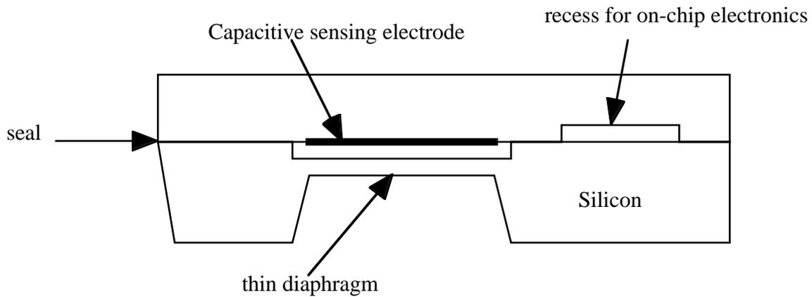
Figure 5. Silicon capacitive pressure sensor
