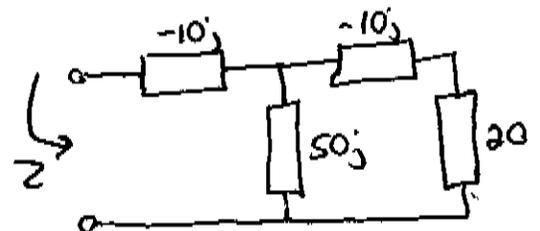
Impedances act like resistors so combine the devices (series or parallel) as if they were resistors.
