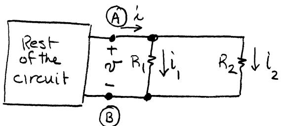
$$\text{KCL @ upper node} \quad \sum_{\text{in}} i = 0 \quad +i - i_1 - i_2 = 0$$
