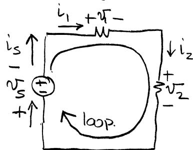
Note source current was aligned with that of loop.
