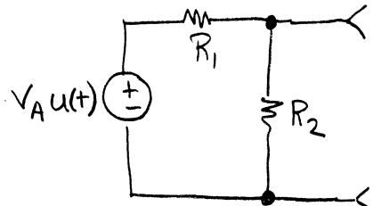
$$V_T = V_{oc} = \frac{R_2}{R_1 + R_2} V_A u(t) = \frac{10k}{30k + 10k} 100 u(t)$$
