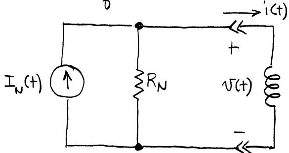
$$I_N(t) = i_{sc}(t) = \frac{R_1}{R_1 + R_2} I_A u(t)$$
