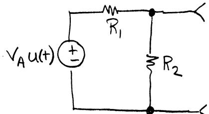
$$V_T = V_{o2} = \frac{R_2}{R_1 + R_2} V_A u(t) = \frac{10k}{30k + 10k} 100 u(t)$$
