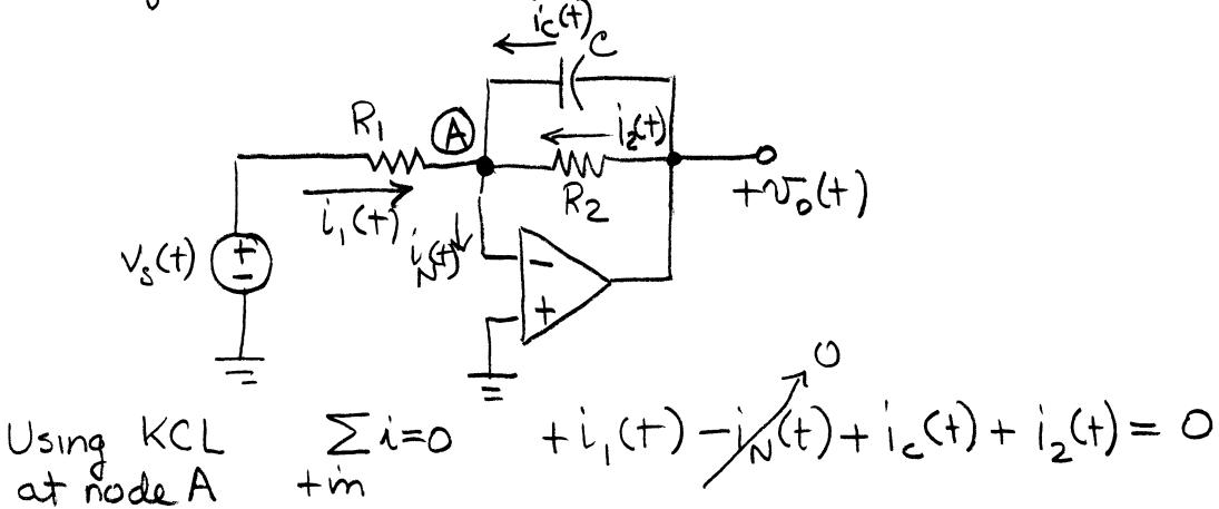
$$\frac{V_s - 0}{R_1} + 0 + C \frac{d}{dt} (v_o - 0) + \frac{v_o - 0}{R_2} = 0$$
