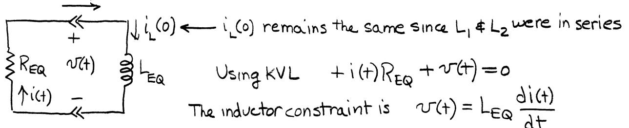
$$\text{Using KVL } +i(t)R_{EQ} + v(t) = 0$$
