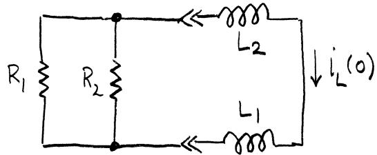
The inductors are in series and can be replaced by an equivalent  $L_{EQ}$ .
