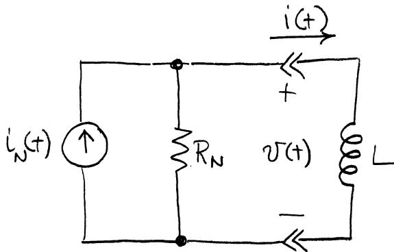
The differential equation is  $\frac{L}{R_N} \frac{di(t)}{dt} + i(t) = I_A$  for  $t \geq 0$
