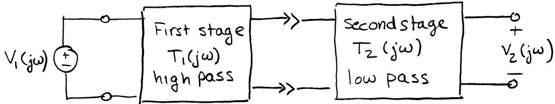
$$T(j\omega) = T_1(j\omega) \times T_2(j\omega)$$
