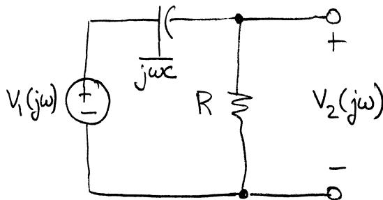
Using voltage division  $V_2(j\omega) = \frac{R}{R + \frac{1}{j\omega C}} V_1(j\omega)$
