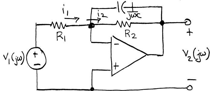
Do KCL at inverting input. Voltage at inverting input is 0 volts,
