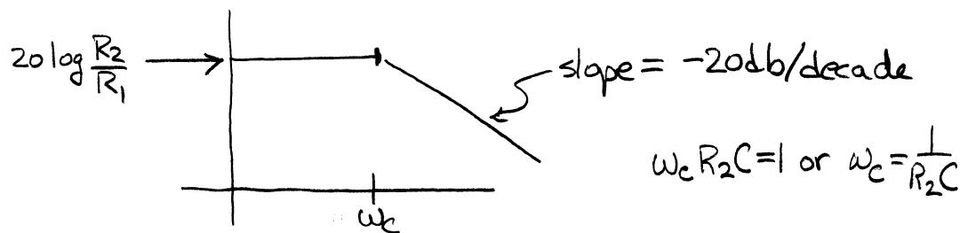
$$\omega_c R_2 C = 1 \text{ or } \omega_c = \frac{1}{R_2 C}$$
