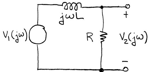
$$\text{Using voltage division } T(j\omega) = \frac{V_2(j\omega)}{V_1(j\omega)} = \frac{R}{R+j\omega L} = \frac{1}{1+j\frac{\omega L}{R}}$$
