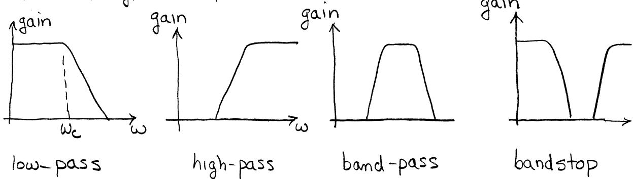
The sinusoidal steady-state output is given by the gain function  $|T(j\omega)|$  and the phase function  $\Theta(\omega)$ .
