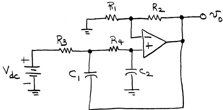
Since this is a dc circuit we replace the capacitors by open circuits and solve.
