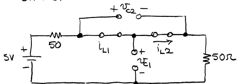
This is basically a two resistor series circuit.
