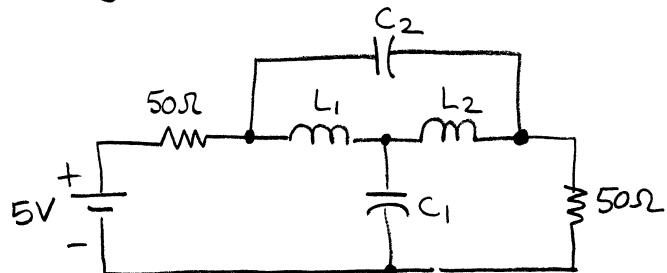
This is a DC circuit analysis. The capacitors are open since they are fully charged. The inductors are correspondingly shorts.
