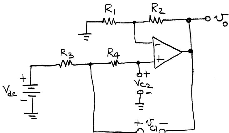
There is no current  $i_p$  into the OP AMP so there are no voltage drops across either  $R_3$  or  $R_4$ .  $\Rightarrow V_p = V_{dc}$
