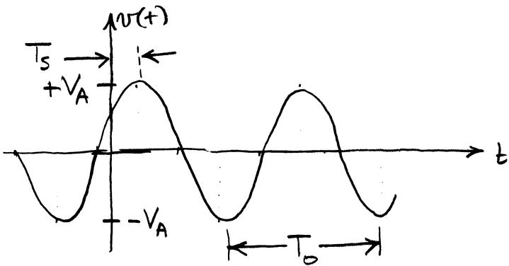
$$v(t) = V_A \cos \left[ 2\pi \left( \frac{t-T_s}{T_0} \right) \right]$$
