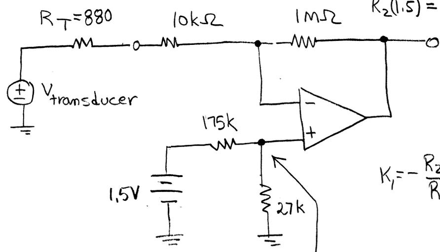
$$K_1 = -\frac{R_2}{R_1} = -\frac{1M\Omega}{10k\Omega} = -100$$
