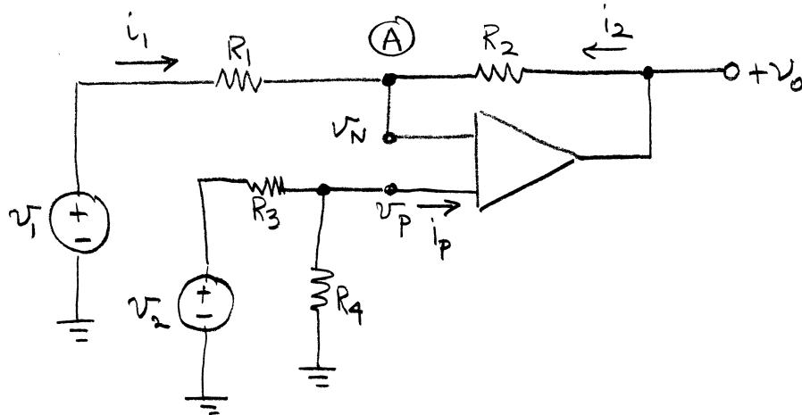
Since  $i_p = 0$      $v_p = \frac{R_4}{R_3 + R_4} v_2$     which is the voltage at A
