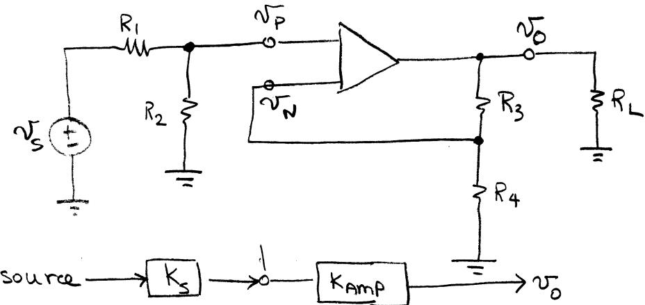
Break circuit into two parts: (1)  $K_s$ , the proportionality constant of the source circuit
