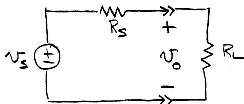
There would be a voltage divider relationship between the input and output circuits.
