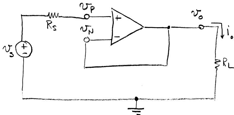
Consider the above circuit where there is a direct connection from the output back to the input.
