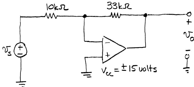
This is an inverting amplifier where  $K = - \frac{33k}{10k} = -3.3$
