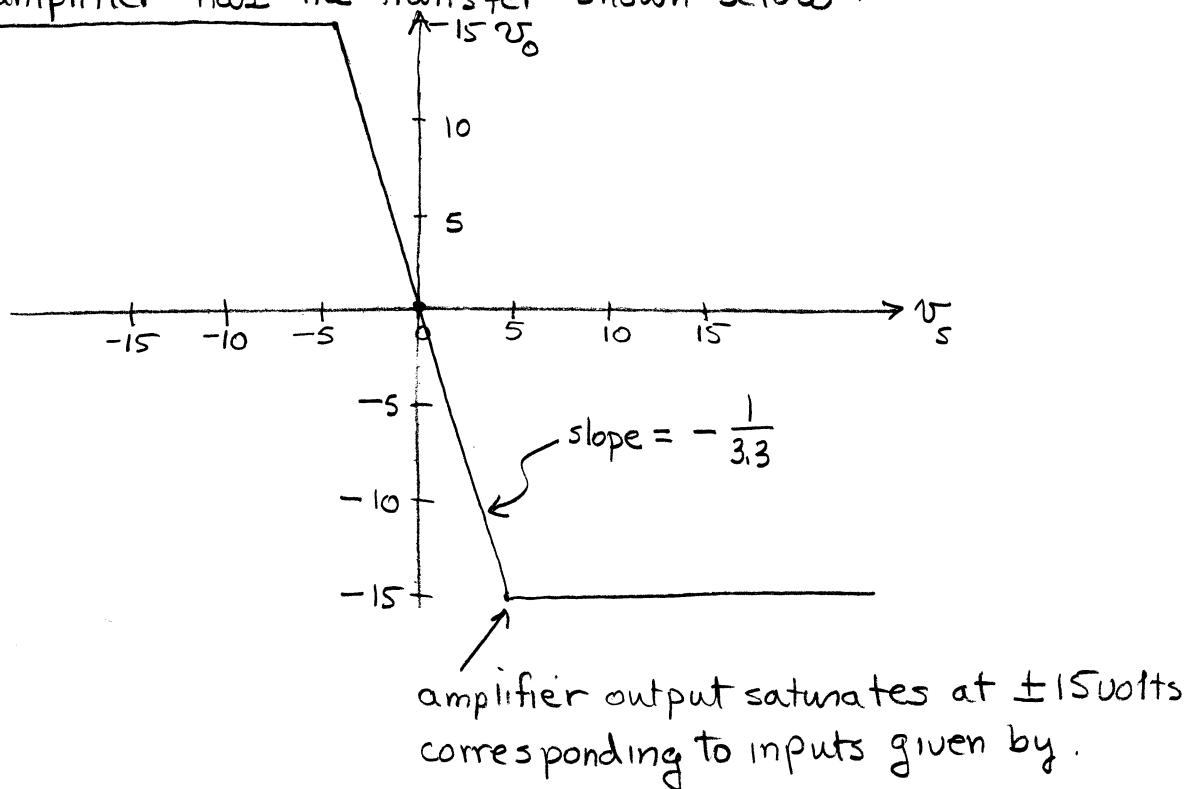
amplifier output saturates at  $\pm 15$  volts corresponding to inputs given by .
