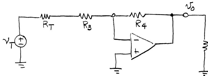
$$\text{where } v_T = \frac{R_2}{R_1 + R_2} v_s$$
