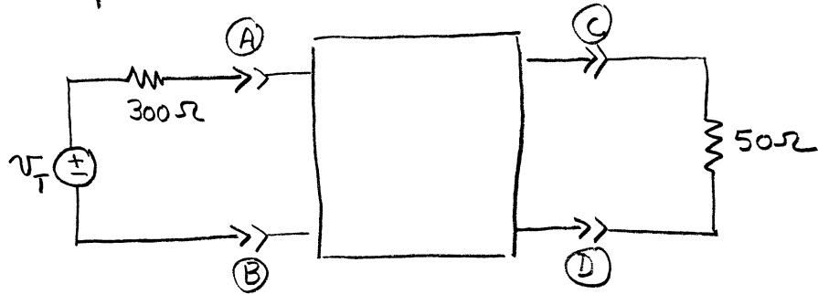
Design the two-port interface circuit so the load "sees" a Thevenin resistance of  $50\Omega$  between terminals  $\textcircled{C}$  and  $\textcircled{D}$ , while simultaneously the source "sees" a load resistance of  $300\Omega$  between  $\textcircled{A}$  and  $\textcircled{B}$ .
