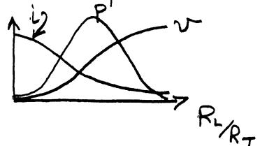
Consider the power being delivered to the load.
