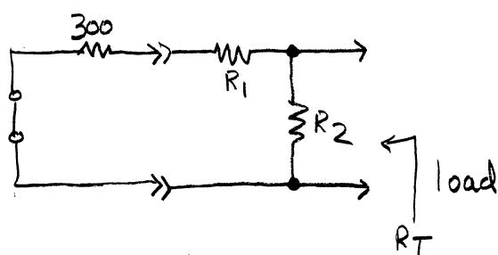
Want load to see a  $R_T$  smaller than source so there has to be a parallel resistance.
