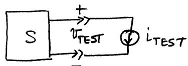
apply a current source  $i_{TEST}$
