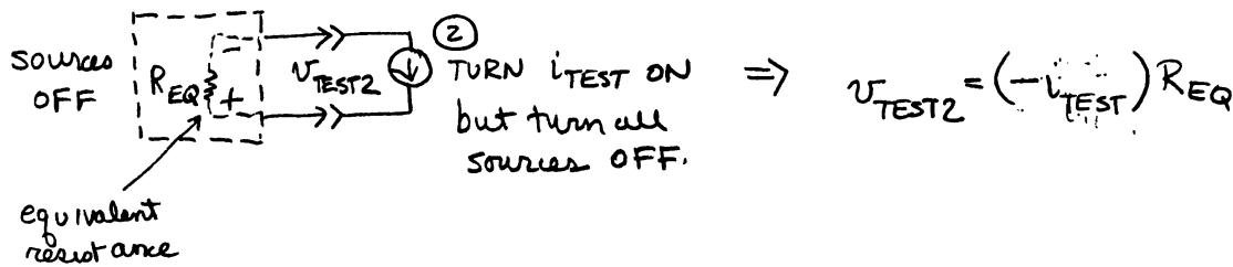
using superposition the sum of ① and ② must be  $v_{TEST}$
