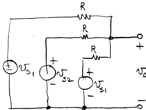
Turn off  $v_{s2}$  and  $v_{s3}$ .
