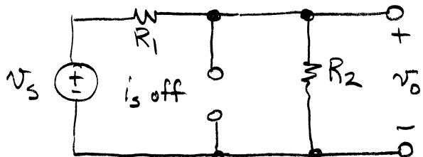
$i_s$  becomes an "open" and the circuit is a voltage divider.
