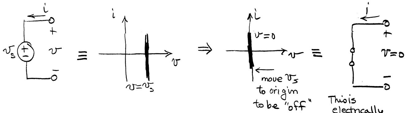
Turning "off" an independent voltage source means replacing it by a short.
