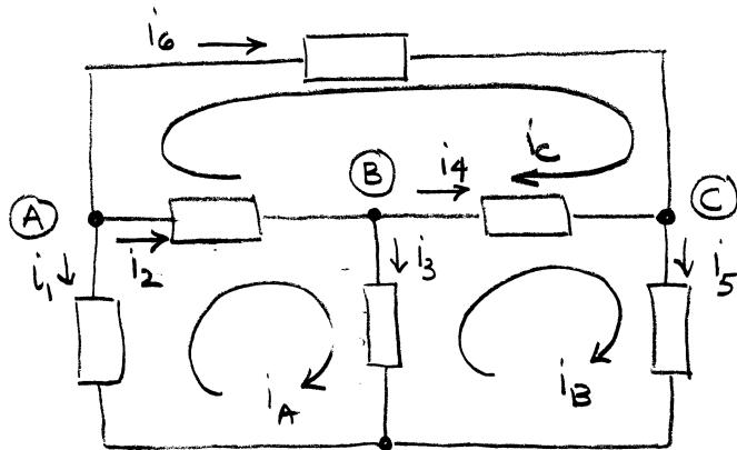
$$\text{By inspection} \quad \left. \begin{array}{l} i_6 = i_c = -3\text{ A} \\ i_5 = i_B = 5\text{ A} \\ i_1 = -i_A = -10\text{ A} \end{array} \right\} \text{outside elements have only one current}$$
