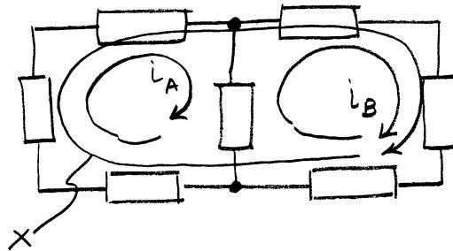
in this drawing  $i_A, i_B$  form meshes; but  $X$  is only a loop because it encloses an element
