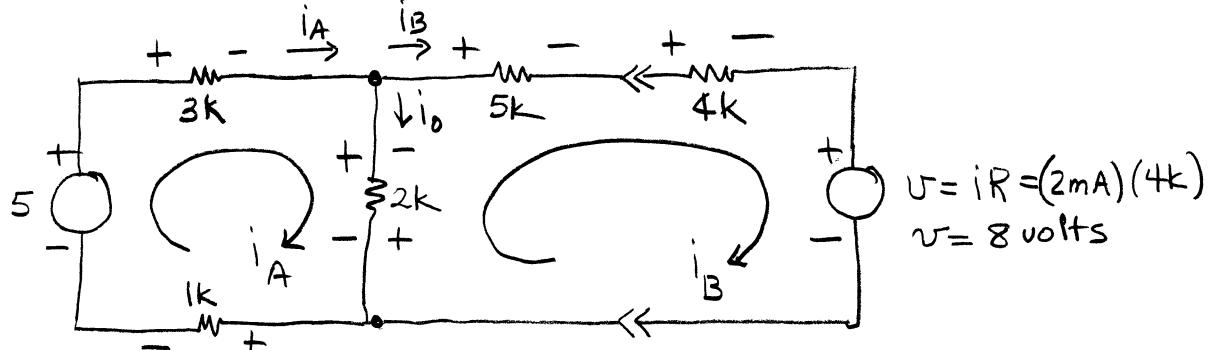
$$\text{KVL for mesh A: } -5 + 3000i_A + 2000i_A - 2000i_B + 1000i_A = 0$$
