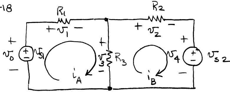
$$\text{mesh A: } \sum_{\text{C1}} V = -v_s 1 + v_1 + v_3 = 0$$
