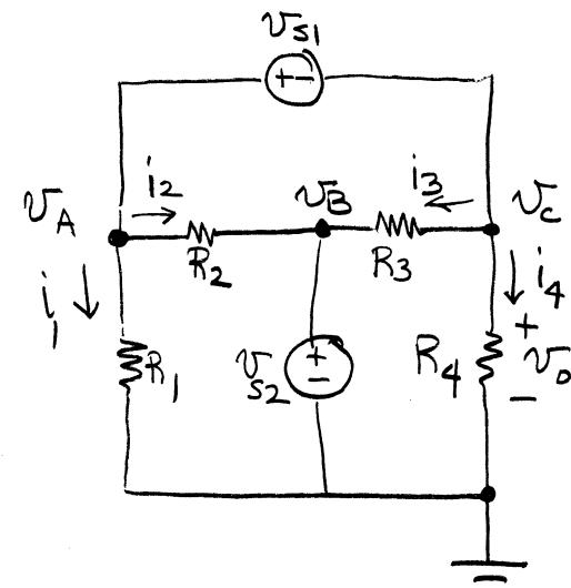
This circuit cannot be solved since we cannot write a current for  $v_A$  or  $v_C$  through  $v_{S1}$ . We cannot use a source transformation on  $v_{S1}$  since it does not have a series resistance. We also cannot ground either node A or C since that would change the circuit. Therefore, we must use a "supermode".
