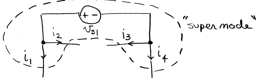
$$\text{For a supermode } \sum_{\text{out}} i = 0 \quad i_1 + i_2 + i_3 + i_4 = 0$$
