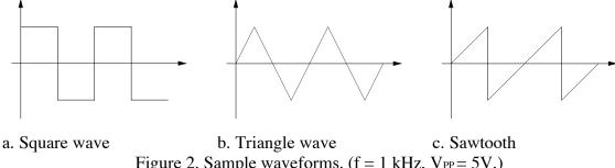
Figure 2. Sample waveforms. (f = 1 kHz,  $V_{PP}$  = 5V.)
