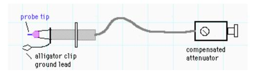
Figure 6. A typical oscilloscope probe
