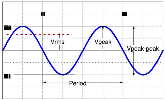
Figure 1. Characterization of sinusoidally time varying signal.
