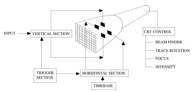
Figure 4 - Functional diagram of oscilloscope
