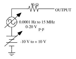
Figure 3 - Functional circuit of a signal generator
