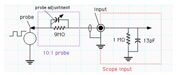
Figure 7. A 10:1 divider network of a typical probe.
