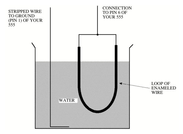
Figure 6. Home made capacitor for water level sensor
