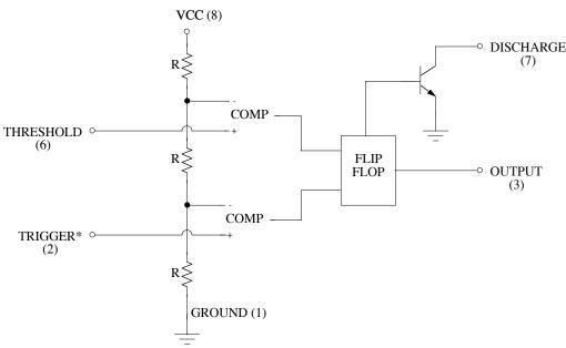
Figure 1. Simplified 555 schematic.
