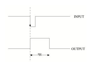
Figure 4. 555 one-shot waveforms
