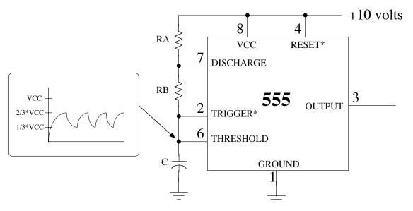
Figure 2. The 555 connected as an oscillator.
