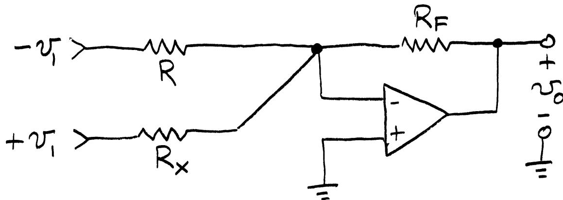
(a) Determine  $\frac{v_o}{v_1}$  for the above circuit.
