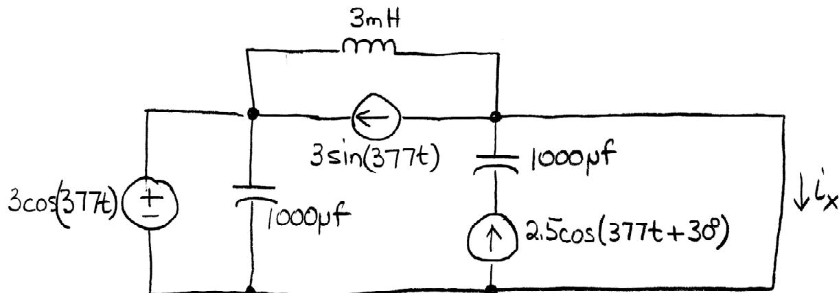
(a) What is the frequency  $f$  in Hertz at which this circuit is operating?  $f = \underline{\hspace{2cm}}$
