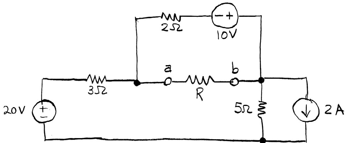
(a) What is the Thevenin equivalent of the circuit as seen by resistor  $R$  at terminals a-b.
