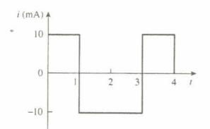
(a) What is the element (inductor or capacitor?) and its numerical value? Capacitor = Q.2mF
