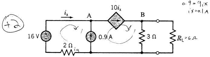
a) Write node analysis equations (KCL) for nodes A and B in terms of  $i_x$  and the given circuit parameters. These are the connection equations. Do not write  $i_x$  in terms of other circuit variables for this part of your answer.
