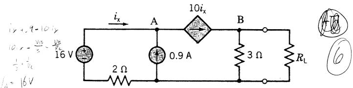
a) Write node analysis equations (KCL) for nodes A and B in terms of  $i_x$  and the given circuit parameters. These are the connection equations. Do not write  $i_x$  in terms of other circuit variables for this part of your answer.
