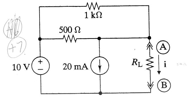
(a) the current  $i_1$  through  $R_L$  from the 10 volts source.  $i_{1=}$
