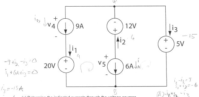
in = (a) Determine the indicated currents through the voltage sources.
