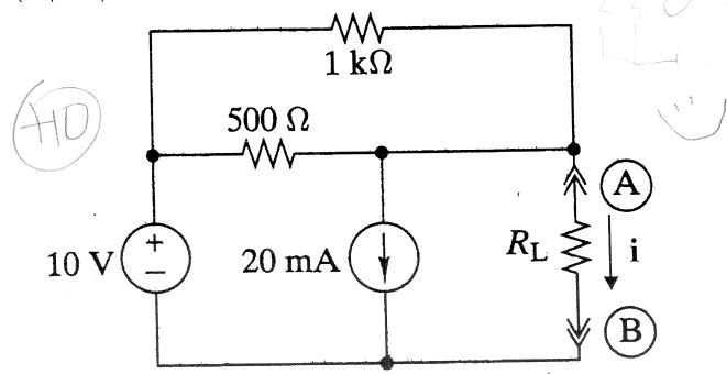
(a) the current  $i_1$  through  $R_L$  from the 10 volts source.  $i_{1=}$  12 m A
