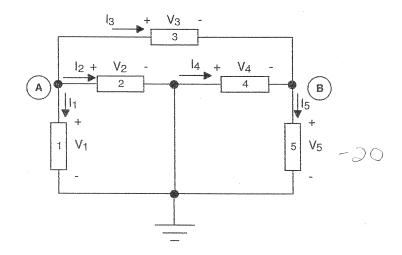
Consider the five element circuit shown above. You measure the electrical parameters shown below for each circuit element. Complete this table and indicate whether each device is absorbing (A) or delivering (D) power. Current is defined to be positive when it flows into the positive terminal of the device.
