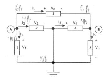
Consider the five element circuit shown above. You measure the electrical parameters shown below for each circuit element. Complete this table and indicate whether each device is absorbing (A) or delivering (D) power. Current is defined to be positive when it flows into the positive terminal of the device.
