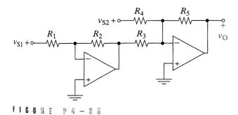
4-31 Find the output  $v_2$  in terms of the input  $v_1$  in Figure P4-31.
