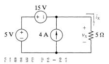
2-22 First use KVL to find the voltage across each resistor in Figure P2-22. Then use Ohm's law and KCL to find the current through every element, including the voltage sources.
