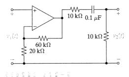
Find the transfer function  $T_{\rm V}(s) = V_2(s)/V_1(s)$  of the circuit in Figure P12-6. What type of gain response does the circuit have? What is the passband gain? Select values of R and C to produce a cutoff frequency of 500 Hz. What is the phase shift at the cutoff frequency?
