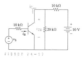
4–18 In Figure P4–18 the transistor parameters are  $\beta=80$  and  $V_{\gamma}=0.7$  V. Find  $i_{\rm C}$  and  $v_{\rm CE}$  for  $v_{\rm S}=1$  V. Repeat for  $v_{\rm S}=4$  V.
