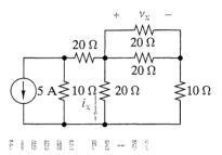
2-52 Use circuit reduction to find  $i_s$  and  $i_x$  in the circuit shown in Figure P2-52.
