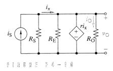
The circuit in Figure P4-11 is a model of a bipolar junction transistor operating in the active mode. The input signal is the current source  $i_{\rm S}$ , and the voltage source  $V_{\rm CC}$  supplies power. Find expressions for the base current  $i_{\rm B}$  and the output voltage  $v_{\rm O}$  in terms of  $V_{\rm CC}$  and  $i_{\rm S}$ .
