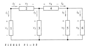
1-23 Figure P1-22 shows an electric circuit with a voltage and a current variable assigned to each of the six devices. The device signal variables are observed to be as follows:
