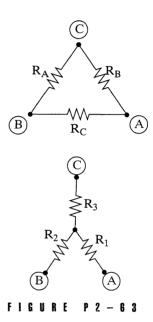
(a) A Show that the two circuits are equivalent when
