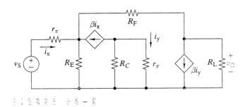
Find an expression for the voltage gain  $v_0/v_s$  in Figure P4–9.
