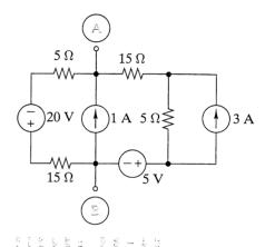
(a) Find the Thévenin or Norton equivalent seen by  $R_L$  in Figure P3–47.
