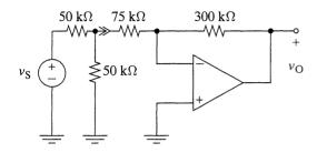
4–22 Find  $v_0$  in terms of  $v_s$  in Figure P4–22.
