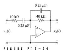
12–15 Find the transfer function  $T_V(s) = V_2(s)/V_1(s)$  of the circuit in Figure P12–15.
