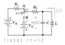
The switch in Figure P7-42 has been in position B for a long time. At t = 0 it is moved to position A. The cir-
