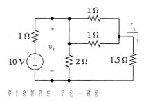
2-54 Use circuit reduction to find  $v_x$  and  $i_x$  in the circuit shown in Figure P2-54.
