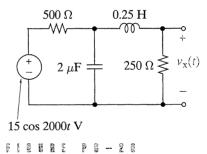
8-27 The circuit in Figure P8-27 is operating in the sinusoidal steady state. Use circuit reduction to find the input impedance seen by the current source and steady-state response  $v_x(t)$ .
