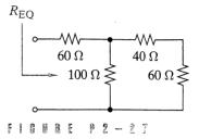
2-28 Find the equivalent resistance  $R_{EO}$  in Figure P2-28.
