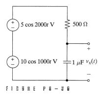
8-31 The circuit in Figure P8-31 is operating in the sinusoidal steady state. Use superposition to find the response  $v_x(t)$ . Note: The sources do not have the same frequency.
