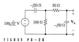
8-29 The circuit in Figure P8-29 is operating in the sinusoidal steady state. Use superposition to find the phasor response  $I_x$ .
