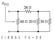
2-29 Find the equivalent resistance  $R_{\rm EQ}$  in Figure P2-29 when the switch is open. Repeat when the switch closed.
