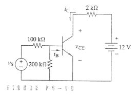
In Figure P4–19 the transistor parameters are  $\beta = 100$  and  $V_{\gamma} = 0.7$  V. Find  $i_{\rm C}$  and  $v_{\rm CE}$ .
