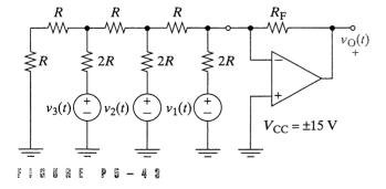
(c) For  $R_F = R$ , use the input-output relationship in (a) and the input timing diagram in (b) to obtain a plot of the output voltage in the range 0 < t < 10 s.
