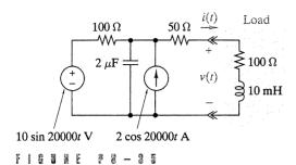
&-36 The circuit in Figure P8-36 is operating in the sinusoidal steady state. When  $Z_L = 0$ , the phasor current at the interface is  $\mathbf{I} = 4.8 - j3.6$  mA. When  $Z_L = -j20$  k $\Omega$ , the phasor interface current is  $\mathbf{I} = 10 + j0$  mA. Find the Thévenin equivalent of the source circuit.
