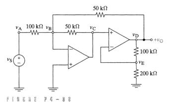
4-34 Find the output  $v_0$  in terms of  $v_1$  and  $v_2$  in Figure P4-34.
