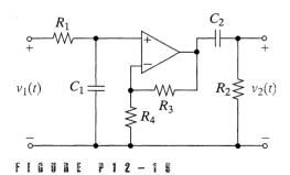
12-20 The transfer function of a bandpass circuit can be written as
