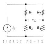
3-24 Use the unit output method to find  $v_0$  in the circuit in Figure P3-24.
