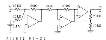
4-32 Find the output  $v_2$  in terms of the input  $v_1$  in Figure P4-32.
