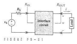
3-62 Figure P3-61 shows a two-port interface circuit connecting source and load circuits. In this problem  $v_S = 15 \text{ V}$ ,  $R_S = 1 \text{ k}\Omega$ , and the load is a diode whose i- $\nu$  characteristic is
