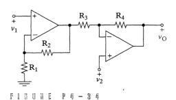
4–35 Find the output  $v_0$  in terms of  $v_1$  and  $v_2$  in Figure P4–35.
