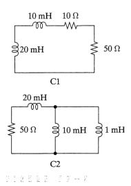
7-6 Find the time constants of the circuits in Figure P7-4.
