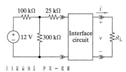
3-70 Design the interface circuit in Figure P3-69 so that the power delivered to the load never exceeds 1 mW regardless of the load resistance.
