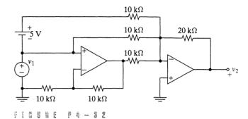
4-33 Find the output  $v_0$  in terms of the input  $v_s$  in Figure P4-33.
