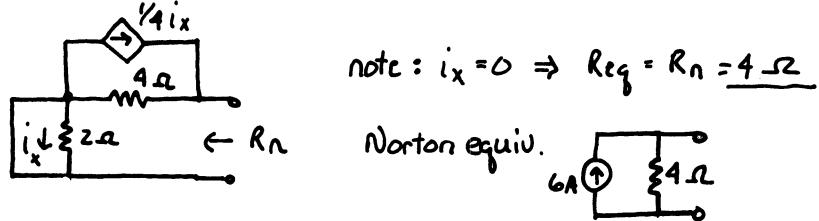
$$\text{note: } i_x = 0 \Rightarrow R_{eq} = R_n = 4 \Omega$$
