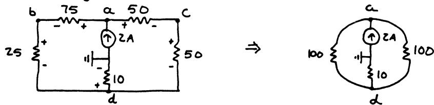
by symmetry 1A flows from a to b & from a to c
