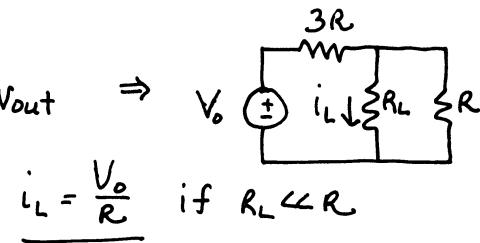
$$\underline{i_L = \frac{V_o}{R}} \quad \text{if } R_L \ll R$$
