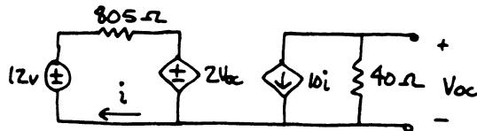
$$\text{KVL around left mesh: } -12 + 805i + 2V_{oc} = 0 \quad (1)$$
