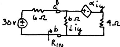
(b) for max power  $R_{IN} = R_T = 6\Omega$
