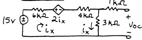
$$\text{KVL } \uparrow i_x : -15 + i_x(6+4) + 2i_x + 3i_x = 0 \\ \Rightarrow i_x = 1\text{mA} \\ \therefore \underline{V_{oc} = 3i_x = 3\text{V}}$$
