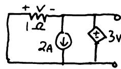
$$\text{KVL: } V + 3V = 0 \\ \Rightarrow V = 0 \\ \therefore V_{oc} = 0$$
