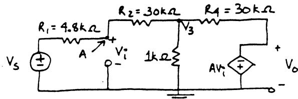
$$\text{KCL at } A : (V_i - V_s)/4.8 = (V_3 - V_i)/30 \Rightarrow V_3 = 7.25V_i - 6.25V_s$$
