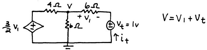
$$\text{KCL at } V: (V - \frac{3}{2}V_1)/4 + V/6 + V_1/6 = 0 \quad \downarrow \text{ with } V = V_1 + 1$$
