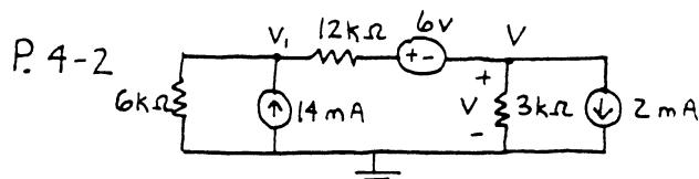
$$\text{KCL at } V_1 : \frac{V_1}{6} - 14 + \frac{(V_1 - 6 - V)}{12} = 0$$
