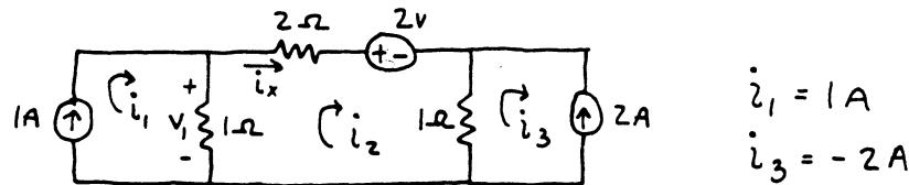
$$\begin{aligned} i_1 &= 1A \\ i_3 &= -2A \end{aligned}$$
