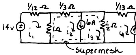
$$\text{mesh (1)}: -14 + \frac{1}{12}i_1 + 1(i_1 - i_2) = 0 \quad (1)$$
