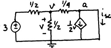
$$\text{KCL at } V: \frac{V-3}{1/2} + \frac{V}{1/2} + \frac{V}{1/4} = 0 \\ \Rightarrow V = \frac{3}{4}V$$
