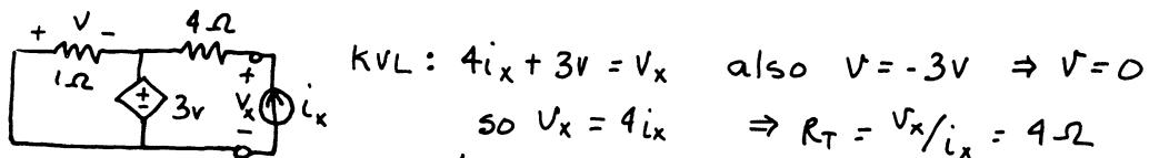
$$\text{KVL: } 4i_x + 3V = V_x \quad \text{also } V = -3V \Rightarrow V = 0 \\ \text{so } V_x = 4i_x \quad \Rightarrow R_T = V_x/i_x = 4\Omega$$
