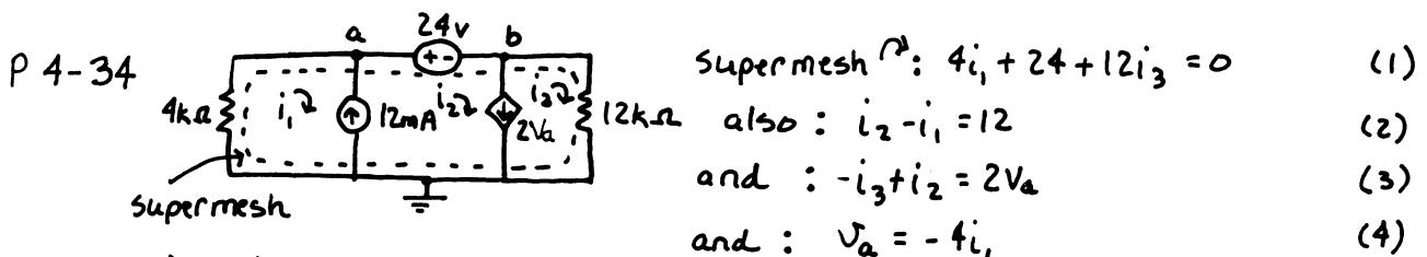
$$\text{Supernode mesh : } 4i_1 + 24 + 12i_3 = 0 \quad (1)$$
