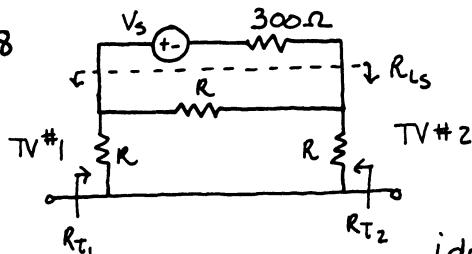
For maximum power to each TV, require  $R_{t1} = 300\Omega$ ,  $R_{t2} = 300\Omega$ . Furthermore, for the source (antenna) to deliver maximum power, we require  $R_{ls}$  (seen by antenna) =  $300\Omega$ . Note that calculation of  $R_{ls}$ ,  $R_{t1}$ ,  $R_{t2}$  leads to identical circuits, hence consider  $R_{t2}$  (kill  $V_s$ )
