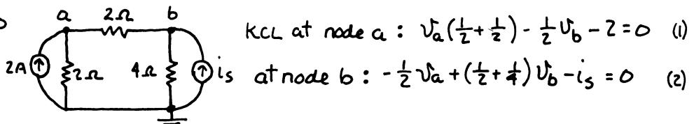
$$\text{now } V_{ba} = 3 = V_b - V_a \Rightarrow V_b = 3 + V_a \quad (3)$$
