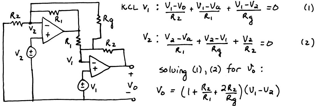
let  $R_g = 200\text{k}\Omega$ ,  $R_2 = 50\text{k}\Omega$  then have  $10 = \left(1 + \frac{50}{R_1} + \frac{100}{200}\right)$
