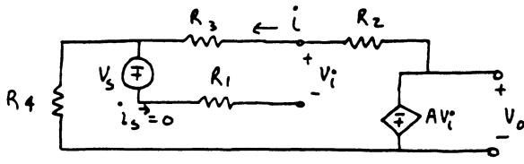
$$\begin{aligned} \text{since } i_s = 0, \text{ from KVL} \\ -V_s - V_i + R_3 i = 0 \\ \Rightarrow i = (V_s + V_i)/R_3 \quad (1) \end{aligned}$$
