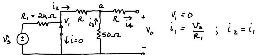
$$\text{at a : } V_a = V_i - i_2 R = -i_2 R = -\frac{V_s R}{R_1}$$
