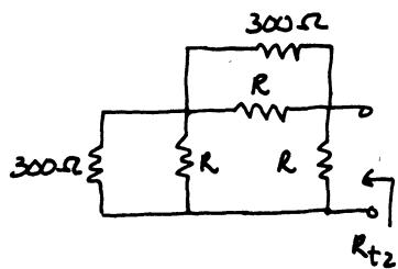
$$\begin{aligned} R_{t2} &= R // \left[ (300//R) + (300//R) \right] \\ &= \frac{2R}{R + R300/R + 300} = 300 \\ \Rightarrow R &= 600 \Omega \end{aligned}$$
