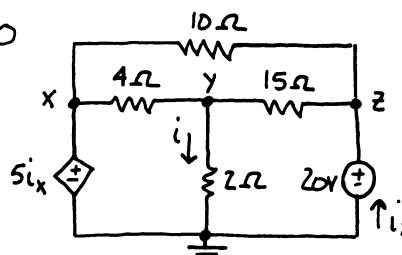
$$\text{by inspection: } V_x = 5i, V_z = 20v, i = \frac{V_y}{2}$$
