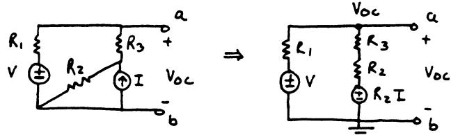
$$\text{KCL at } V_{OC}: \frac{(V_{OC}-V)}{R_1} + \frac{(V_{OC}-R_2 I)}{R_2+R_3} = 0$$
