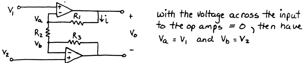
$$\therefore \text{from KVL} : V_0 - iR_3 - iR_2 - iR_1 = 0 \\ \Rightarrow V_0 = i(R_1 + R_2 + R_3)$$
