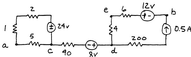
$$\text{KVL around acdeba } \uparrow : V_{ab} = V_{ac} + V_{cd} + V_{de} + V_{eb}$$
