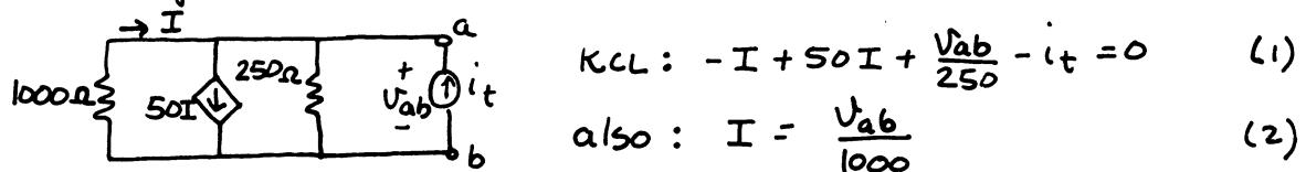
$$(1) \& (2) \text{ yield } i_t = \frac{53}{1000} V_{ab} \quad \text{or} \quad R_{out} = \frac{V_{ab}}{i_t} = \frac{1000}{53} = \underline{18.9\Omega}$$
