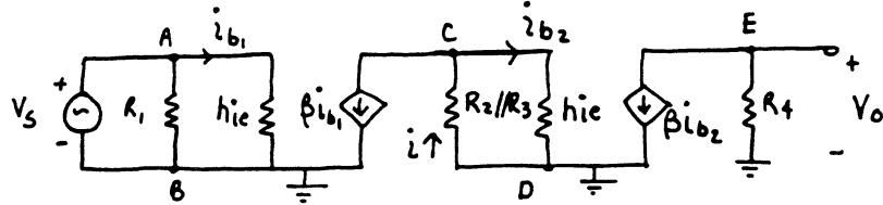
$$\text{KVL around } ABA \text{ loop: } h_{ie}i_{b1} - V_s = 0 \Rightarrow V_s = 1.3i_{b1} \quad (1)$$
