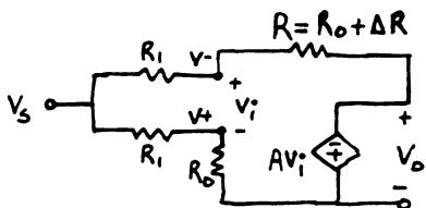
$$\text{from voltage divider: } V_+ = \frac{R_0}{(R_0 + R_1)} V_S \quad (1)$$
