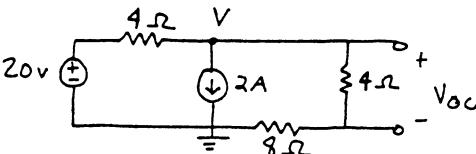
$$KCL \text{ at } V: \frac{(V-20)}{4} + 2 + \frac{V_{oc}}{4} = 0$$
