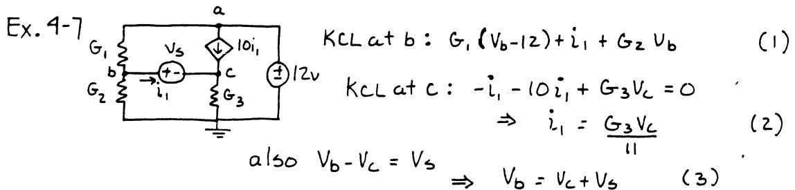
$$\text{KCL at } b : G_1(V_b - 12) + i_1 + G_2 V_b = 0 \quad (1)$$
