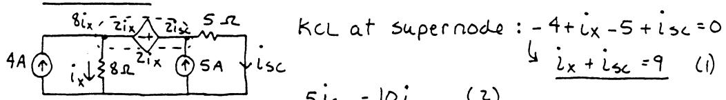
Solving (1) & (2) simultaneously  $\Rightarrow i_{sc} = 6A$
