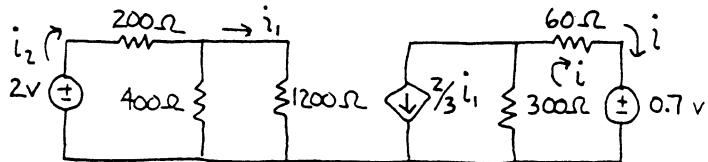
$$\text{from Voltage divider } 1200i_1 = 2 \left( \frac{400/1200}{400/1200 + 200} \right) = 2 \left( \frac{3}{5} \right) = 1.2 \\ \therefore i_1 = 0.001 \text{ A}$$
