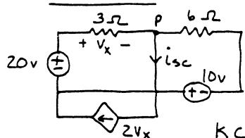
$$\text{KVL left mesh } \uparrow : -20 + V_x = 0 \Rightarrow \underline{V_x = 20\text{V}} \quad (1)$$
