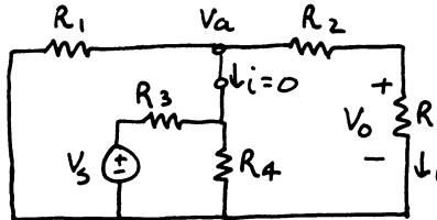
$$V_i = \frac{R_4}{R_3 + R_4} V_s, \quad V_a = V_i = \alpha V_s$$
