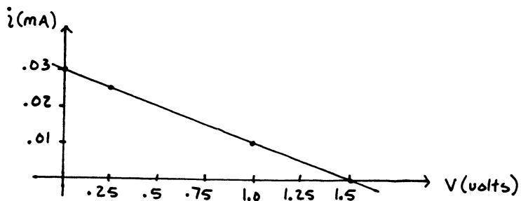
since  $i$  vs  $V$  is linear  $\Rightarrow$  circuit is linear
