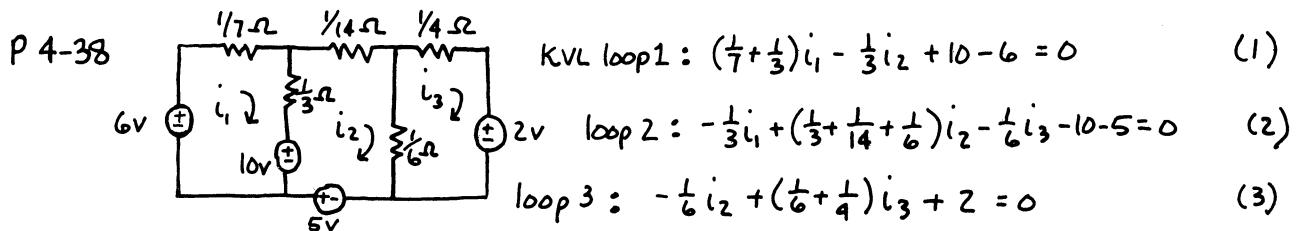
Solving (1) - (3) simultaneously yields  $i_1 = 21A, i_2 = 42A, i_3 = 12A$
