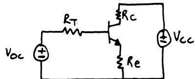
$$\text{where } V_{oc} = V_{cc} \left( \frac{R_2}{R_1 + R_2} \right)$$
