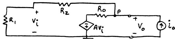
KCL at P:  $i_o - V_o / (R_1 + R_2) - (V_o + A V_i) / R_o = 0 \quad (1)$
