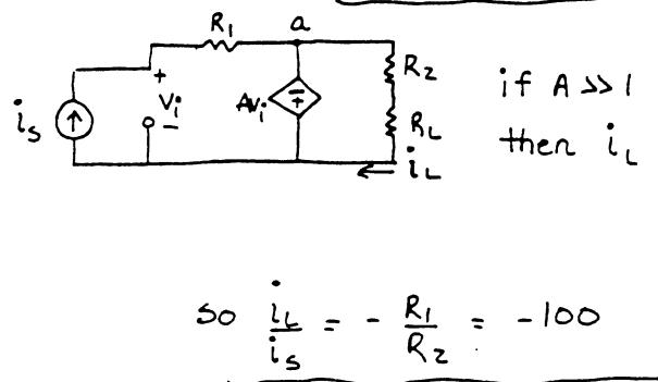
$$\text{if } A \gg 1 \text{ and } V_i = 0 \Rightarrow V_a = -i_s R_1$$
