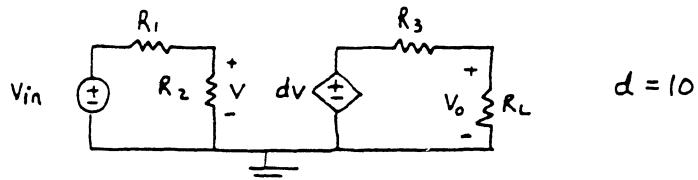
$$\text{from voltage divider } V = \frac{R_2}{R_1 + R_2} V_{in}$$
