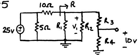
$$R = R_1 \parallel R_2 \parallel (R_3 + R_4)$$
