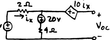
$$\text{KVL around 1st mesh: } -50 + 2i_x - 20 + 4i_x = 0 \Rightarrow i_x = 7.5 \text{ A}$$
