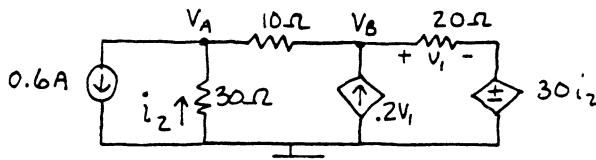
$$\text{KCL at } V_A : 6 - i_2 + \frac{(V_A - V_B)}{10} = 0 \quad (1)$$
