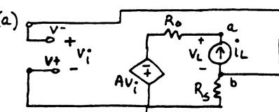
replace  $R_L$  with current source  $i_L$  and find  $R = V_L/i_L$
