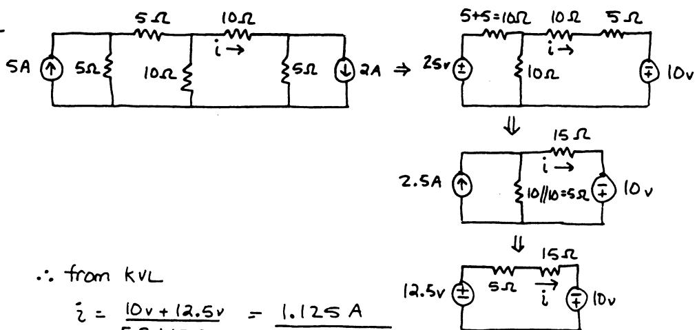
Ex 5-3 Using the method of voltage source transform, we change the two voltage sources into two current sources
