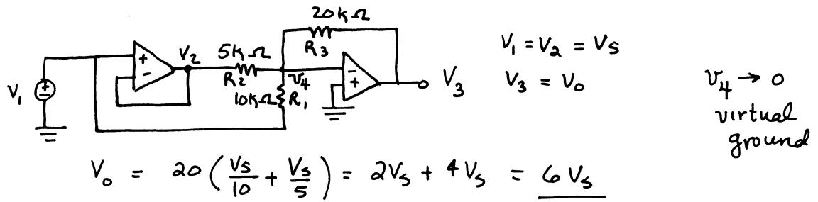
$$\text{since KCL at } V_4 \text{ is } \frac{V_o}{20} = \frac{V_s}{10} + \frac{V_s}{5}$$
