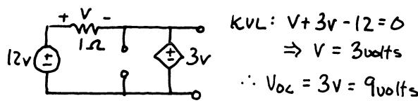
$$\text{KVL: } V + 3V - 12 = 0 \\ \Rightarrow V = 3 \text{ volts}$$
