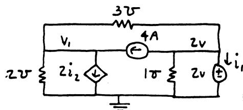
$$\text{KCL at } V_1: 2V_1 + 2i_2 - 4 + i_2 = 0$$
