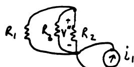
$V''' = 0$  since no current flows through  $R_2, R_3$  and  $R_1$ .
