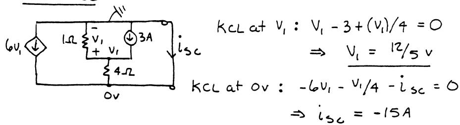
$$\therefore R_T = \frac{V_{oc}}{i_{sc}} = \frac{15}{-15} = -1\Omega \Rightarrow \boxed{\text{Norton equivalent circuit: } 15A \text{ current source in parallel with } -1\Omega \text{ resistor}}$$
