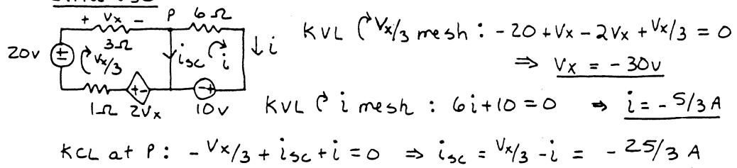
$$\therefore R_T = \frac{V_{oc}}{i_{sc}} = \frac{25}{-25/3} = -3\Omega \quad \text{Thev. equiv. ckt}$$
