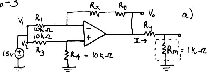
$$V_1 = V_2 = 15 \text{ V} \quad \text{from result of problem 6-1}$$
