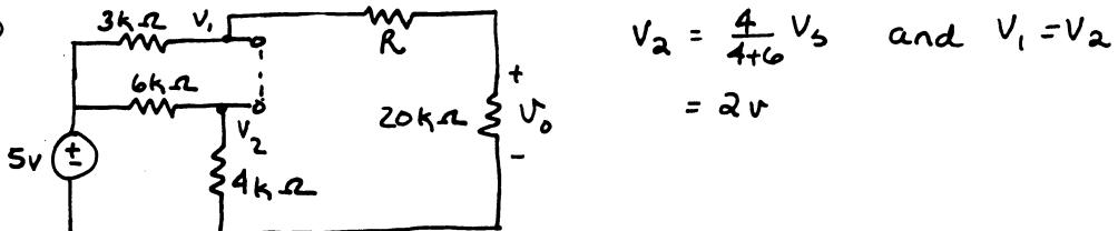
$$V_2 = \frac{4}{4+6} V_s \quad \text{and} \quad V_1 = V_2 \\ = 2V$$
