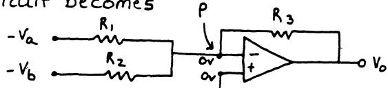
$$\text{KCL at } P: \frac{V_a}{R_1} + \frac{V_b}{R_2} = \frac{V_o}{R_3} \Rightarrow V_o = \frac{R_3}{R_1} V_a + \frac{R_3}{R_2} V_b$$
