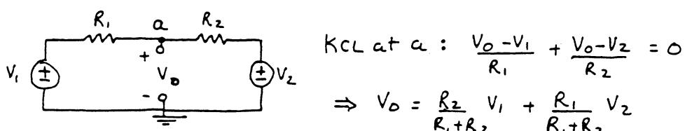
$$\text{KCL at } a : \frac{V_0 - V_1}{R_1} + \frac{V_0 - V_2}{R_2} = 0$$
