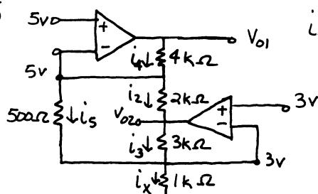
$$i_5 = \frac{5-3}{500} = 4 \text{ mA}, \quad i_X = \frac{3-V_x}{1} \text{ (mA)}$$
