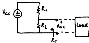
find  $R_T$  : kill  $V_{cc}$  source  $\Rightarrow R_T = R_1 // R_2 = \frac{R_1 R_2}{R_1 + R_2}$
