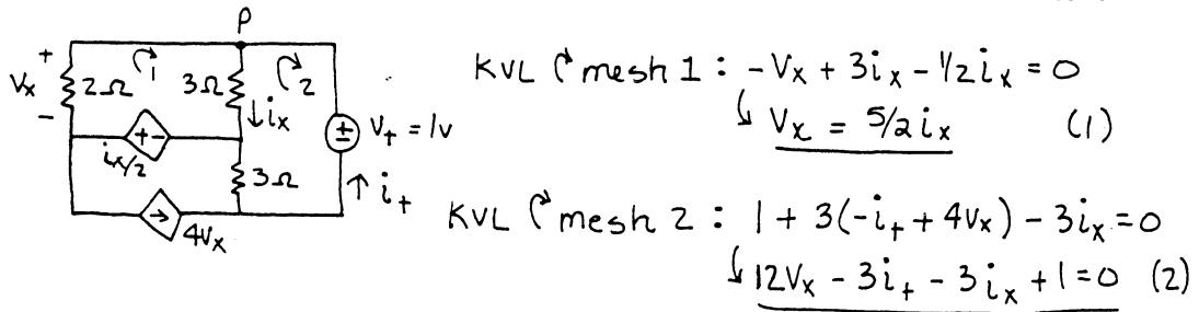
$$KCL \text{ at } P: \frac{V_x}{2} + i_x - i_T = 0 \quad (3)$$
