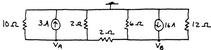
$$\text{KCL at } V_A : \frac{V_A}{10} + 3 + \frac{V_A}{2} + \frac{1}{2}(V_A - V_B) = 0$$
