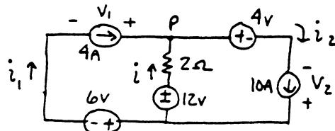
$$\text{KCL at } P: i = i_2 - i_1 \\ i = 10 - 4 = 6 \text{ A}$$
