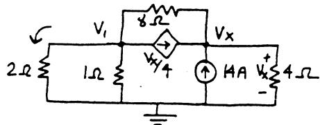
$$\text{KCL at } V_i : \frac{V_i}{2} + \frac{V_i}{1} + \frac{(V_i - V_x)}{8} + \frac{V_x}{4} = 0 \\ \Rightarrow \underline{13V_i + V_x = 0} \quad (1)$$
