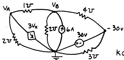
$$\text{KCL at } V_A: 2V_A + 3V_x + V_x = 0$$
