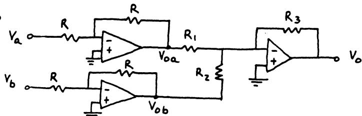
(a) assume ideal op amps  $\Rightarrow V_{oa} = -V_a$  and  $V_{ob} = -V_b$
