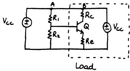
since points A & B are at same potential virtually no current exists between A-B ∴ open ckt.
