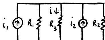
$$\text{where } i_1 = \frac{V_1}{R_1} = -\frac{1}{2}e^{-t} \text{ (A)}$$
