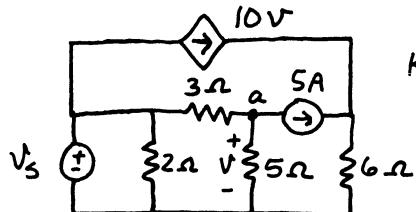
$$\text{KCL at node } a : V\left(\frac{1}{5} + \frac{1}{3}\right) + 5 - \frac{V_s}{3} = 0$$
