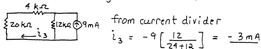
$$\therefore \underline{i = i_1 + i_2 + i_3 = -\frac{1}{3} + \frac{4}{3} - 3 = -2 \text{ mA}}$$
