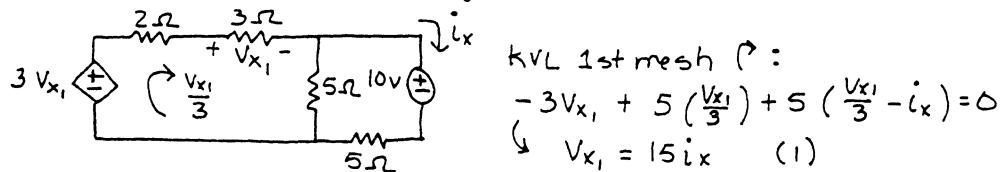
$$\text{KVL 2nd mesh } \uparrow: 5(i_x - V_{x_1}/3) + 10 + 5i_x = 0 \quad (2)$$
