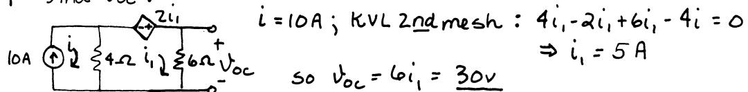
$$\text{so } V_{oc} = 6i_1 = 30V$$
