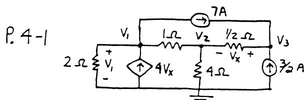
$$\text{KCL at } V_1 : \frac{V_1}{2} - 4V_x + 7 + (V_1 - V_2) = 0 \Rightarrow \underline{3V_1 - 2V_2 - 8V_x + 14 = 0} \quad (1)$$
