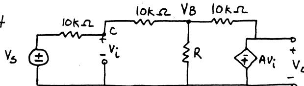
$$\text{KCL at } C : (V_i - V_s)/10 + (V_i - V_B)/10 = 0 \Rightarrow V_B = 2V_i - V_s \quad (1)$$
