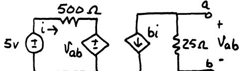
$$\text{find } i_{sc} : V_{ab} = 0 \quad \therefore i = 5/500 = 10mA$$
