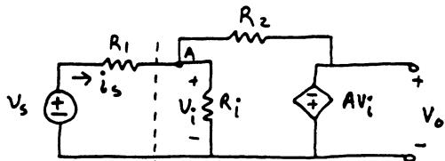
← find the Thévenin equiv. to right of dotted line and add  $R_T$  to  $R_1$  to get total  $R_{IN} = V_s/i_s$
