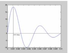
The book gives the period of the sine wave to be 5ms, the value of the first peak to be at 18V at 1.3ms, and the value of the first minimum to be at -10V. The u(t) means that the value of this function at times less than t=0 is 0V.
