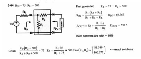
The best way to solve these design problems is to try each Interface Circuit equivalent shown in Figure 3-52 on pg. 118 of the text. Since this is a design problem you can guess some values and use logic into which is the best interface circuit to use for specifications required.
