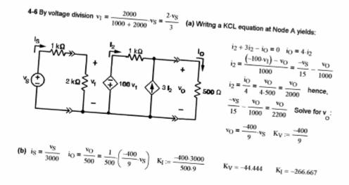
Therefore,  $\underline{Kv} = -44.44$  for part (a); and  $\underline{K_I} = -266.667$  for part (b)
