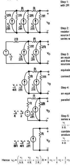
Step 1: Convert the voltage sources in series with 2R to equivalent current sources in parallel
