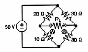
Finding the equivalent "lookback" resistance or Thevenin resistance is quite hard to visualize but if you rearrange the circuit drawing enough you can clearly see that  $10\Omega \parallel 20\Omega$  which is in series with the  $30\Omega \parallel 30\Omega$ . Therefore,
