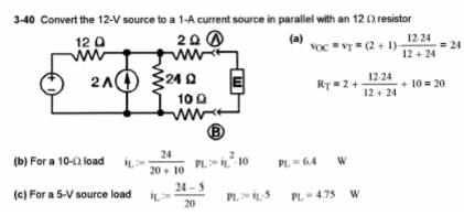
Remember to open the circuit at A and B, and use superposition to solve for Voc
