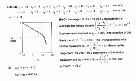
(d) The model says that  $v_{OC} = 15 \text{ V}$  whereas the data  $(v_0)$  says  $v_{OC} = 12 \text{ V}$ . The model only applies to the range -10 V < v < +10 V because the characteristic is nonlinear for v > 10 V
