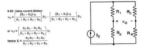
Consider the current through the resistor and the voltage drops at each resistor, an easy way to look at this problem is to consider is as dividing the current in parallel with  $(R1 + R3) \parallel ((R2 + R4))$ . Then, there is a voltage division between, R1 and R3; R2 and R4. This gives you a better concept of the behavior of the circuit. Solve in terms of Vo/Is.
