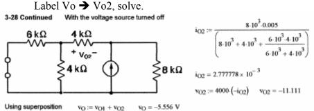
**Step 3:** Hence, if Vo = Vo1 + Vo2, simply added the two together, and you have found the voltage across the 4k $\Omega$  resistor. <u>Vo = -5.556 V</u>
