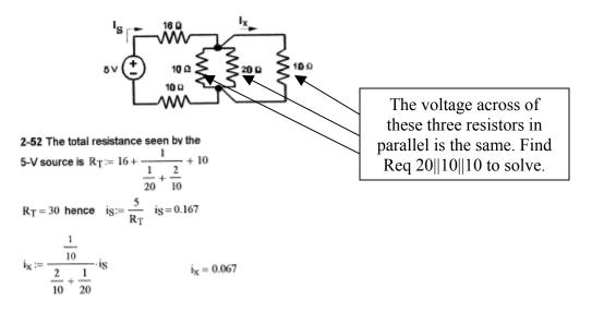
After considering the 3 resistors in parallel to be an equivalent resistance, find the voltage drops across the remaining resistor that are is series. After finding the voltage drop across the Req simply use Ohms law to find current Ix = 0.067.
