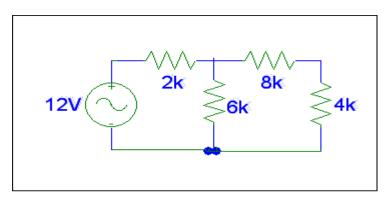
First reduce circuit to find the voltage at the node after the  $2k\Omega$  resistor. First add together  $8 k\Omega$  and  $4 k\Omega$  resistors because they are in series which is  $12 k\Omega$ . Now consider the  $6 k\Omega$  resistor to be in parallel with the  $12 k\Omega$  resistor:
