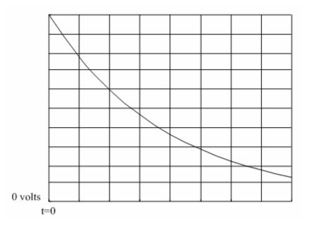
(a) You are in the laboratory measuring an exponential waveform with your oscilloscope. If the units are 20 mS/div horizontal and 8 volts/div vertical determine the numerical value of the time constant Tc for the following waveform.
