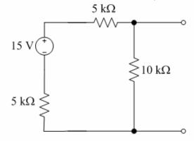
(4) Combine two resistors together;  $5 \text{ k}\Omega + 5 \text{ k}\Omega = 10 \text{ k}\Omega$ ;
