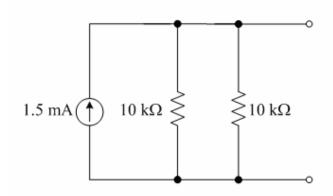
(6) Combine two resistor together; 10 k $\Omega$ //10 k $\Omega$ =5 k $\Omega$ ;
