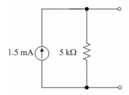
(7) Convert 1.5 mA in parallel with 5 k $\Omega$  to 7.5 V in series with 5 k $\Omega$ ;
