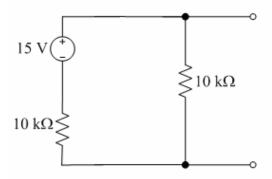
(5) Convert 15 V in series with 10 k $\Omega$  to 1.5 mA in parallel with 10 k $\Omega$ ;
