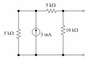
(3) Convert 3 mA in parallel with 5 k $\Omega$  to 15 V in series with 5 k $\Omega$ ;
