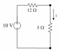
So we can easily calculate the current through the 5  $\Omega$  resistor:
