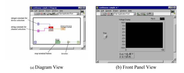
Figure 6. Sample VI that Reads Channel 0 from Device 1
