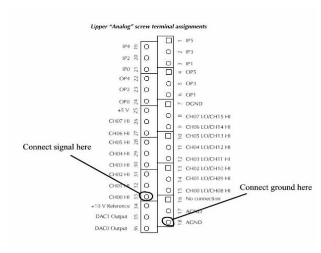
Figure 8. Analog screw terminal assignments
