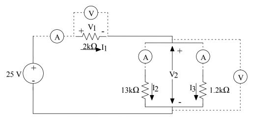
Figure 11. Current divider circuit.
