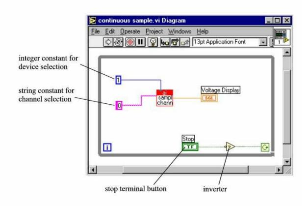
Figure 1. LabVIEW Program to Read a Voltage from a Single Channel and Display that Voltage Value on a Waveform Chart.
