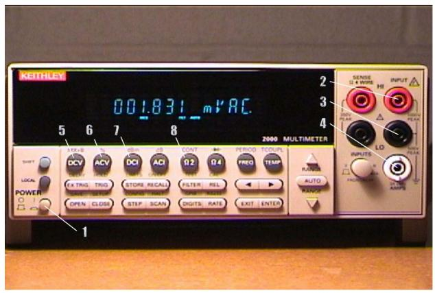
Figure 9. Keithley Model 2000 Multimeter
