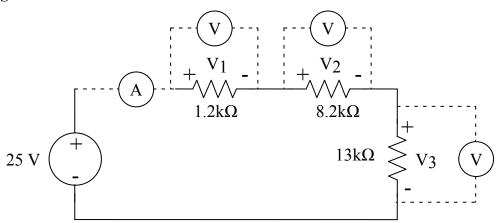
Figure 10. Voltage divider circuit.
