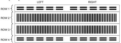
Figure 3. Solderless breadboard
