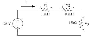
Figure 4. Voltage divider circuit.
