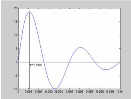
The book gives the period of the sine wave to be 5ms, the value of the first peak to be at 18V at 1.3ms, and the value of the first minimum to be at -10V. The  $u(t)$  means that the value of this function at times less than  $t=0$  is 0V.
