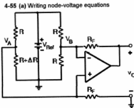
Node A:  $\left(\frac{1}{R} + \frac{1}{R + \Delta R} + \frac{1}{R_f}\right)v_A - \frac{v_{Ref}}{R} = 0$
