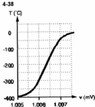
At -300 °C the transducer output is 1.006 mV and the desired output is 0 V. At -100 °C the transducer output is 1.00667 mV and the desired output is +5 V.
