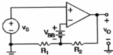
(a)  $v_P = v_S \quad v_N = \left( \frac{R_1}{R_1 + R_2} \right) \cdot v_O + V_{BB}$
