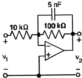
We can evaluate the transfer function using the formula for the gain of an OP AMP amplifier and recognizing that the 5nF capacitor and the 100kΩ resistor are in parallel.
