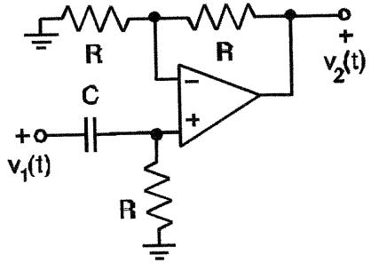
You can recognize this as a subtractor circuit by comparing it with Figure 4-40 of Thomas and Rosa. However, it is probably easiest to analyze by simply computing the voltages at the two inputs assuming an ideal OP AMP and then setting the inputs equal. Both input voltages are given by voltage divider relationships as
