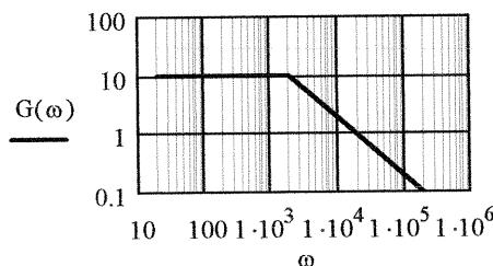
(c ) The output voltage for a particular input voltage and frequency is simply the phasor magnitude of the input voltage times the gain expression evaluated for the frequency of the input, i.e.,  $V_o(\omega) = G(\omega) \times 5$
