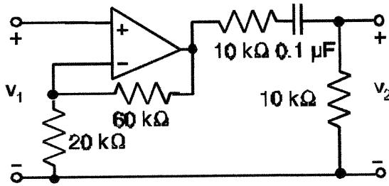
This is an interesting problem because it consists of a amplifier and a separate filter. The OP AMP amplifier produces a voltage at its output node which is then modified by the output voltage divider. This can be written as the product of the amplifier gain times the output voltage divider as shown below:
