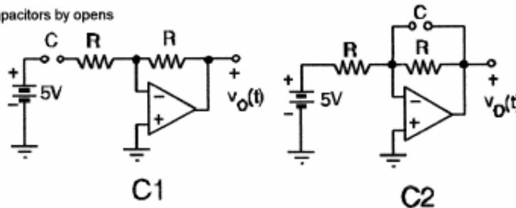
For C1 when C is open the source and OP AMP are disconnected hence  $v_O := 0$  V
