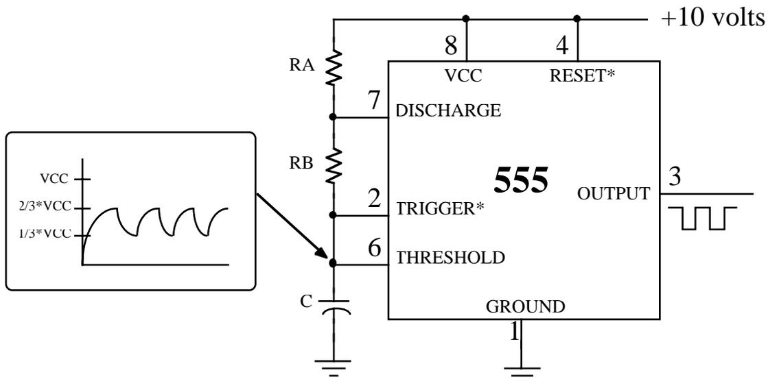
**Figure 2. The 555 connected as an oscillator.**
