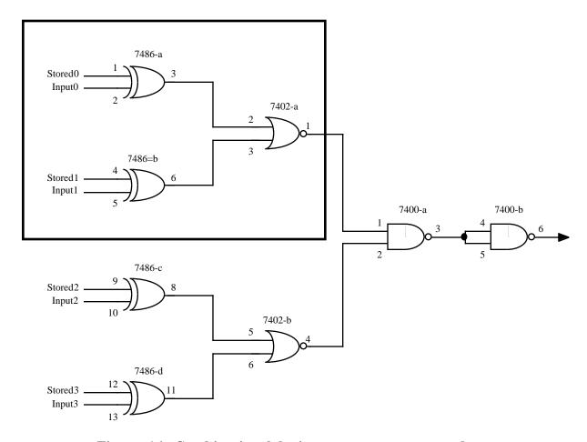
Figure 16. Combinational logic to compare two numbers.
