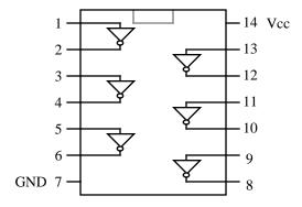
Figure 3. A 7404 integrated circuit (IC) contains 6 inverters.
