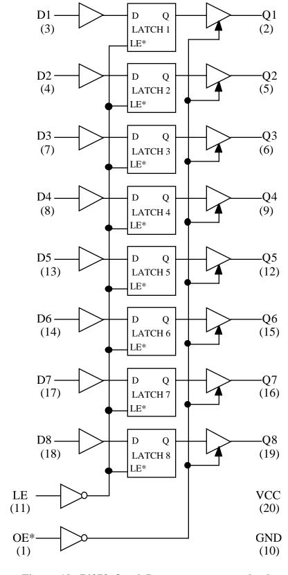
Figure 12. 74373 Octal D-type transparent latch
