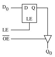
Figure 10. Logic diagram of D-latch.
