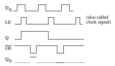
Figure 11. Timing diagram of D-latch. (Note that  $Q_0$  is undefined when OE\* is high.)
