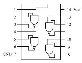
Figure 5. A 7400 IC contains 4 2-input NAND gates.
