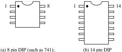
Figure 1. Physical configuration of 8 and 14 pin DIP IC devices.
