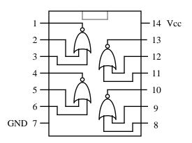
Figure 7. A 7402 IC contains 4 2-input NOR gates.
