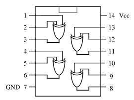
Figure 9. A 7486 IC contains 4 2-input XOR gates.
