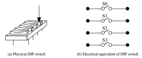
Figure 17. DIP (Digital Inline Package) Switch
