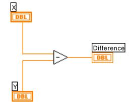
Figure 1-6. Subtract Operation in LabVIEW®
