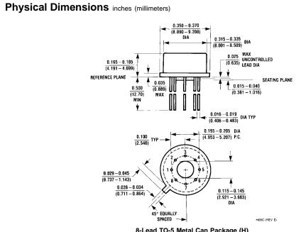
8-Lead TO-5 Metal Can Package (H) Order Number LMC555CH NS Package Number H08C
