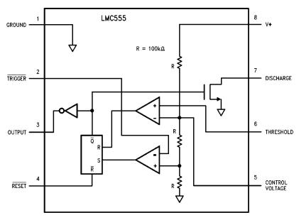
(Pinouts for Molded and Metal Can Packages are identical)
