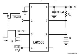
$t_{H}$  = 1.1 R<sub>A</sub>C (Gives time that output is high following trigger)
