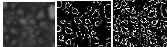
Figure 3a, b and c. The left image is the original, center is the result of CED with Gaussian smoothing, and right is the result of CED without Gaussian smoothing.
