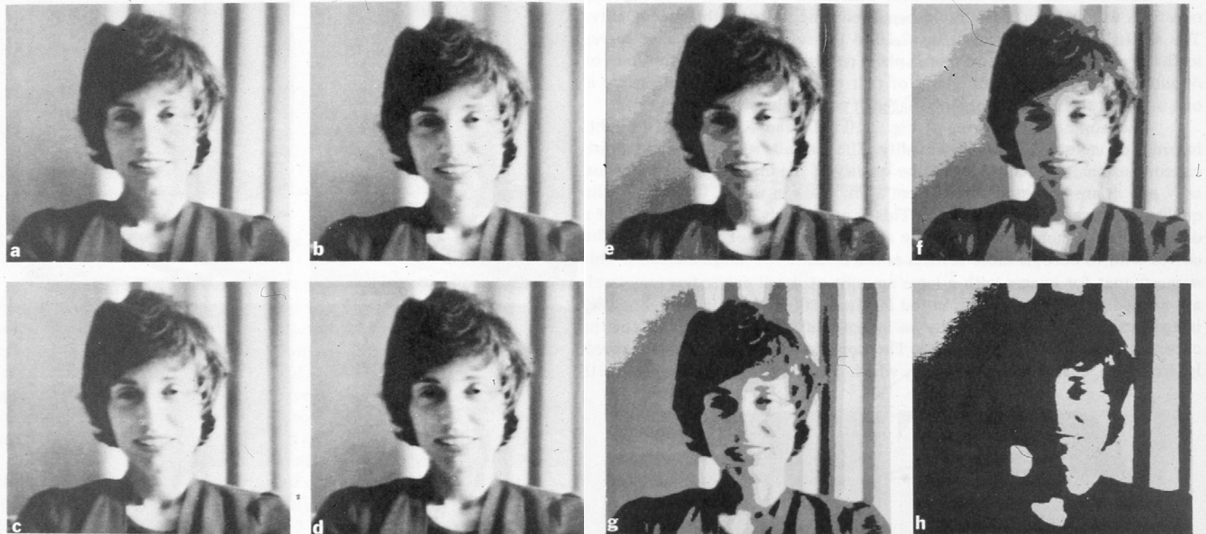
Figure 2.8. A 512 \times 512 image displayed in 256, 128, 64, 32, 16, 8, 4, and 2 levels, respectively.
