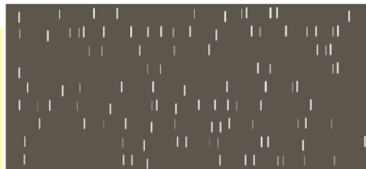
FIGURE 9.29 (a) Text image of size 918 \times 2018 pixels. The approximate average height of the tall characters is 50 pixels. (b) Erosion of (a) with a structuring element of size 51 \times 1 pixels. (c) Opening of (a) with the same structuring element, shown for reference. (d) Result of opening by reconstruction.
