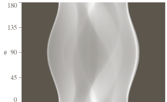
FIGURE 5.39 Two images and their sinograms (Radon transforms). Each row of a sinogram is a projection along the corresponding angle on the vertical axis. Image (c) is called the Shepp-Logan phantom . In its original form, the contrast of the phantom is quite low. It is shown enhanced here to facilitate viewing.
