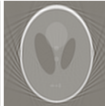
FIGURE 5.47 Reconstruction of the head phantom image from filtered fan backprojections. (a) 1^\circ increments of \alpha and \beta . (b) 0.5^\circ increments. (c) 0.25^\circ increments. (d) 0.125^\circ increments. Compare (a) with Fig. 5.44(b).
