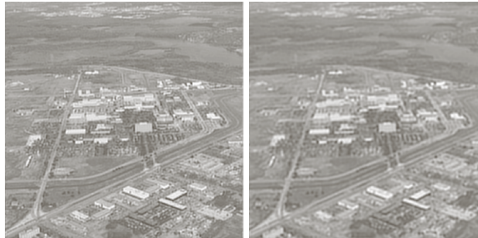
FIGURE 5.31 (a) Iteratively determined constrained least squares restoration of Fig. 5.16(b), using correct noise parameters. (b) Result obtained with wrong noise parameters.
