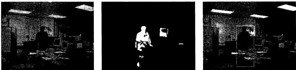
Figure 9.1 (left) A person appears in a formerly unoccupied workspace; (center) image subtraction reveals changed regions where the person occludes the background and at the door and a CRT; and (right) the change due to the person is deemed significant while the other two are expected and hence ignored. (Images courtesy of S.-W. Chen.)
